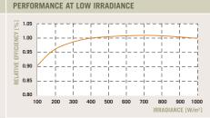
The typical change in module efficiency at an irradiance of 200 W/m² in relation to 1000 W/m² (both at 25 °C and AM 1.5 G spectrum) is -4 % (relative).
